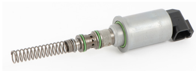
EHPV mechanical feedback couples the pilot and piloted elements to increase position accuracy and response.
