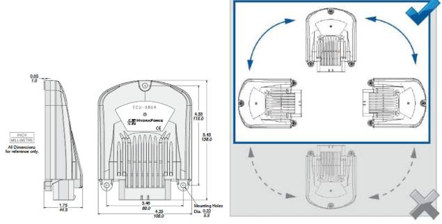
**Note:** When mounting the ECU-0809, be sure to mount with the plug facing down or to the side. Do not mount the unit in a position where the connector side is facing up.
