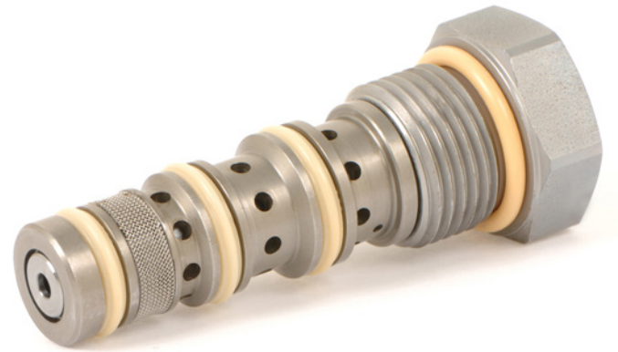
This 4-way 2-position valve halves the inlet pressure to balance torque between series motors in a drive circuit.
